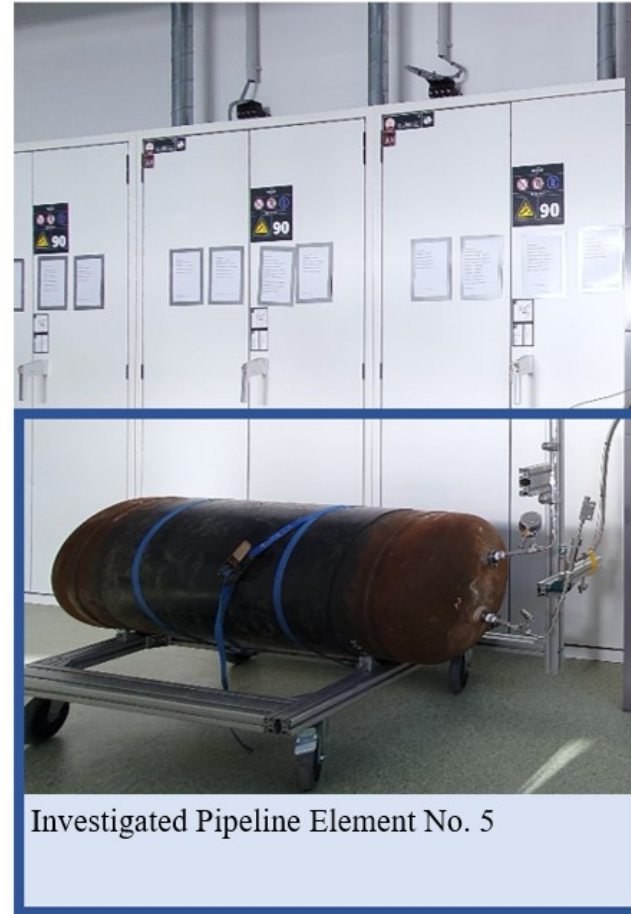
Measurement Setup at HyCentA Boltzmann Lab (IMR-MS, bottom right; FTIR, up right)
